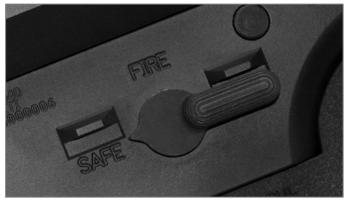
Ensure that the firearm is pointed in a safe direction and that the safety selector is on "SAFE."
