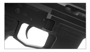
Eject the magazine by depressing the magazine release button.
