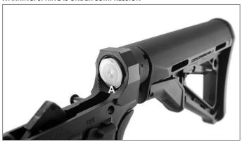
Press down on the buffer retainer (A) while holding the buffer back. Allow the buffer to travel forward slowly after clearing the retainer.
