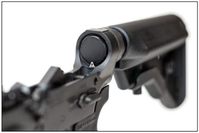
Press down on the buffer retainer (A) while holding the buffer back. Allow the buffer to travel forward slowly after clearing the retainer.
