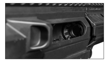
Pull the charging handle to the rear. Visually and physically inspect the firearm by looking inside the ejection port and verifying that there are no cartridges in the chamber.
