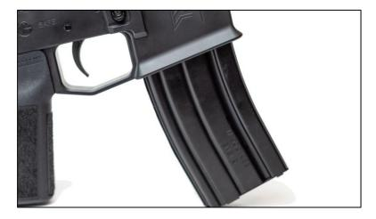
Insert the magazine into the magazine well and ensure that it is properly seated in the firearm. The gun can be loaded with an open or closed bolt.
