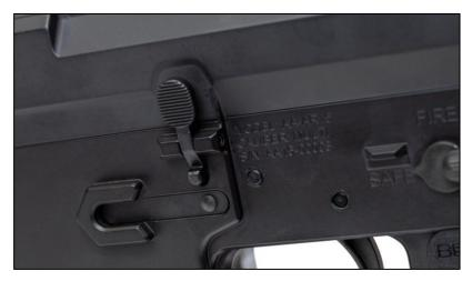
Pull the charging handle all the way to the rear and press the bottom portion of the bolt catch. Release the charging handle. This locks the bolt in the open position.
