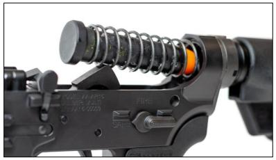
Once the spring is no longer compressed, remove the buffer from the buffer tube.
