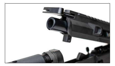
Unlatch the charging handle and pull back. Pull the bolt carrier group straight back until it's free of the upper receiver and charging handle.
