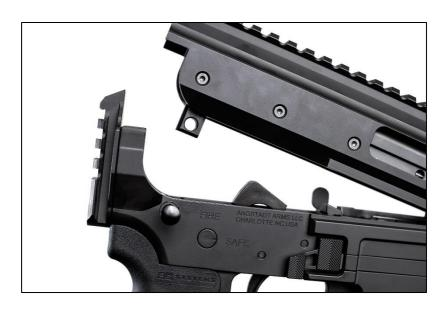
Grasp the upper receiver and pull upward, allowing it to pivot forward.
