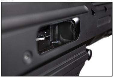
Pull the charging handle to the rear. Visually and physically inspect the firearm by looking inside the ejection port and verifying that there are no cartridges in the chamber.
