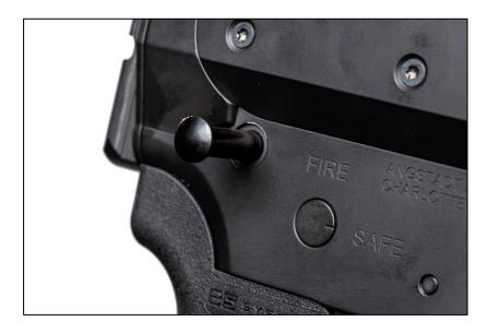
Push in the takedown pin and pull the pin from the right side of the receiver until it stops.
