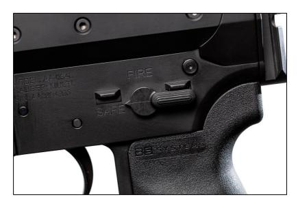
Point the firearm in a safe direction and place the safety selector on "SAFE."
