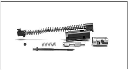
Pull out the firing pin retaining pin. Once removed, stand the bolt carrier on end and the firing pin and spring should fall out of the back of the bolt carrier. While holding the carrier, rotate the bolt 90 degrees clockwise. Due to fouling, it may be necessary to use a pair of pliers to turn the bolt. Slide the bolt forward and remove the slider from the bolt carrier
