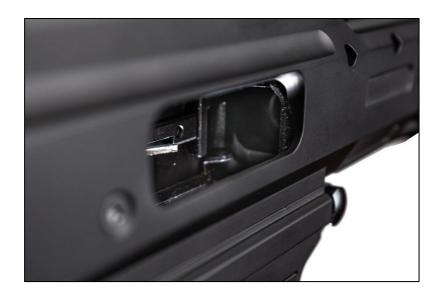
Visually and physically inspect the firearm by looking inside the ejection port and verifying that there are no cartridges in the chamber.
