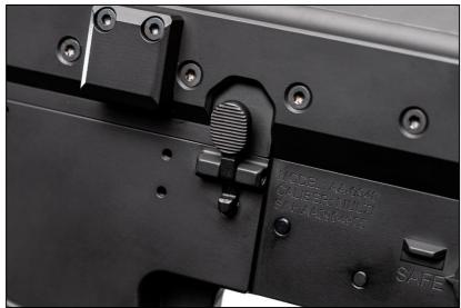
Pull the charging handle all the way to the rear and press the bottom portion of the bolt catch. Release the charging handle. This locks the bolt in the open position.
