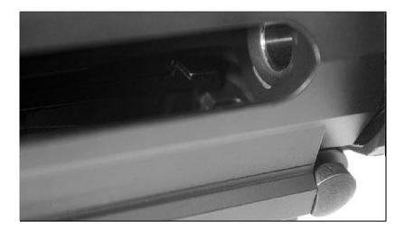
Visually and physically inspect the firearm by looking inside the ejection port and verifying that there are no cartridges in the chamber.
