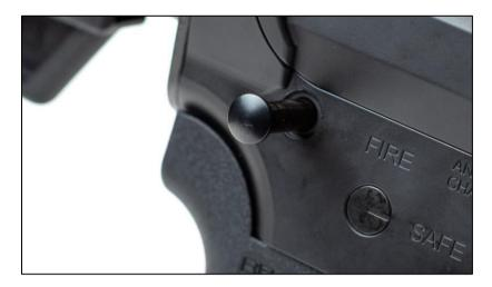
Push in the takedown pin and pull the pin from the right side of the receiver until it stops.
