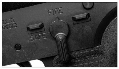
Carefully pull the trigger. The firearm will discharge and automatically load another cartridge into the chamber. The firearm is now ready to be fired again. The process will repeat each time the trigger is pulled. When the last cartridge has been discharged, the bolt will lock open and remain in the rearward position.
