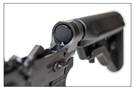
Once the spring is no longer compressed, remove the buffer from the buffer tube.
