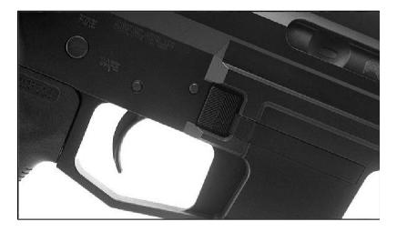
Eject the magazine by pressing the magazine release button.
