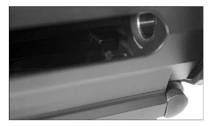
Pull the charging handle to the rear. Visually and physically inspect the firearm by looking inside the ejection port and verifying that there are no cartridges in the chamber.
