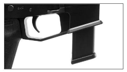
Insert the magazine into the magazine well and ensure that it is properly seated in the firearm. We recommend loading the gun with an open bolt.
